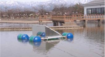
For this location, one Solar powered Rotary Nanobubble generator (equivalent to 50 A/S unit), was installed. It was anticipated that the trial would cover an area of 20m radius. e.g.  $20 \text{ m} \times 20 \text{ m} \times 3.14 = 1,256 \text{ m}^2$
