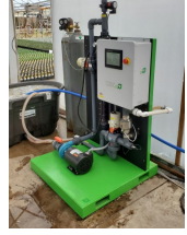
Grower uses Nanobubbles injected with CO2 on the leaves of the plants to increase CO2 uptake
